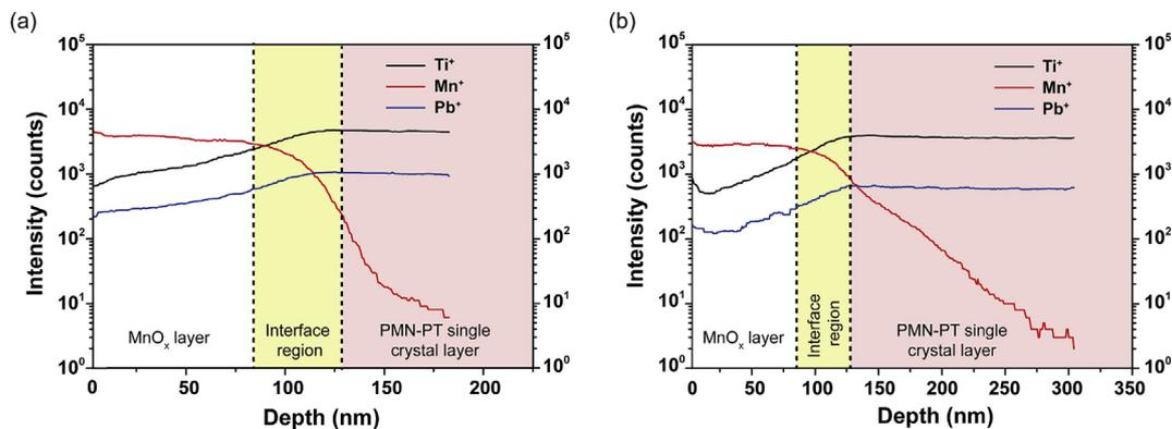
Fig. 3. ToF-SIMS results of  $\text{MnO}_x$  nanocomposite electrodes with and without heat treatment (a) PMN-PT without heat treatment; (b) PMN-PT after heat treatment.
