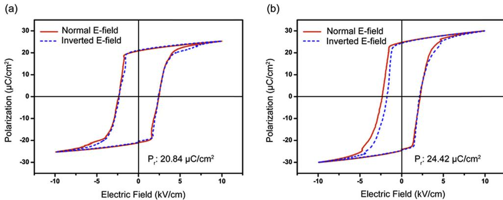
**Fig. 7.** Normal and inverted electric field (E-field) induced ferroelectric (P–E) hysteresis loop. (a) PMN-PT with conventional planar electrodes. (b) PMN-PT with nanocomposite electrodes on one surface and a plane electrode on the other surface.
