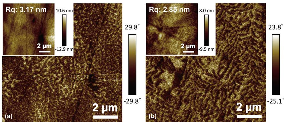
Fig. 4. The PFM domain image of PMN-PT with conventional planar electrodes in different thicknesses. (a) The thickness of the sample is 30  $\mu\text{m}$ , and (b) 200  $\mu\text{m}$ ; the insert images are the topography and surface roughness.
