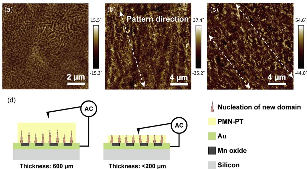
Fig. 5. The PFM domain image result of PMN-PT with  $\text{MnO}_x$  nanocomposite electrodes in different thicknesses. (a) 600  $\mu\text{m}$  (b) 200  $\mu\text{m}$  (c) 30  $\mu\text{m}$  (d) schematic images of nucleation of new domain observation by PFM for samples in different thickness.
