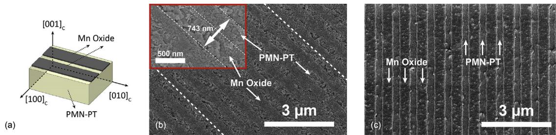
**Fig. 1.** The schematic and SEM image of fabrication results. (a) The  $\text{MnO}_x$  nanograting was fabricated parallel to  $[010]_c$  direction (b) the  $\text{MnO}_x$  nanograting pattern on PMN-PT single crystal surface, (c) it shows the clear  $\text{MnO}_x$  nanocomposite electrodes after 100 nm gold electrode deposition.
