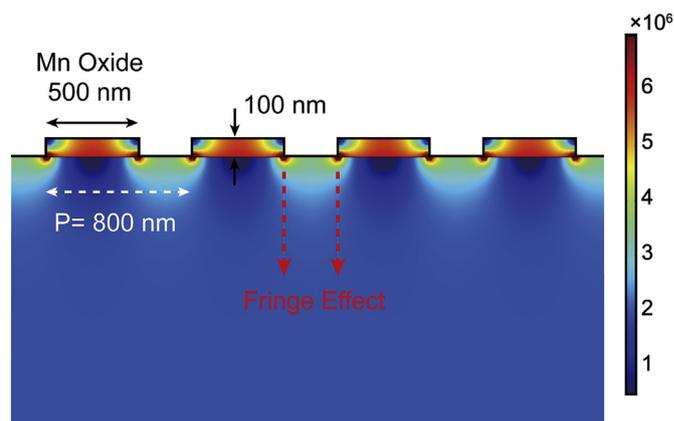
**Fig. 2.** The fringe effect simulation of  $\text{MnO}_x$  nanocomposite electrode. The  $\text{MnO}_x$  nanograting has an  $800 \text{ nm}$  period with pattern size  $500 \text{ nm}$  and  $100 \text{ nm}$  in width and thickness, respectively. The color bar denotes the electric field intensity. (For interpretation of the references to colour in this figure legend, the reader is referred to the web version of this article.)
