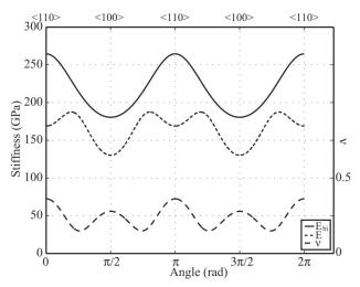
Fig. 3.  $E_{\rm bi}$ , E, and  $\nu$  of silicon as functions of angle from the  $\langle 110 \rangle$  direction within the (110) plane.
