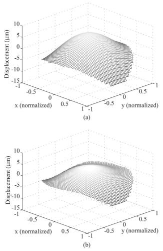
Fig. 6. Measured back wafer surface profile of a (110) silicon wafer (a) before and (b) after deposition of a 20 nm thick Cr film.
