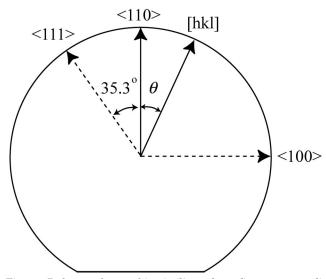
Fig. 2. Reference frame of (110) silicon plane. Some common directions are labeled.
