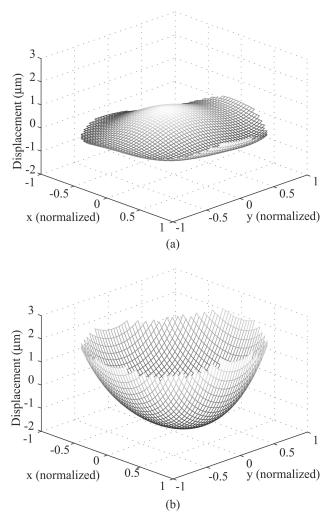
Fig. 5. Measured back wafer surface profile of a (100) silicon wafer (a) before and (b) after deposition of a 20 nm thick Cr film.
