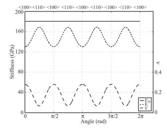
Fig. 1.  $E_{\rm bi}$ , E, and  $\nu$  of silicon as functions of angle from the  $\langle 100 \rangle$  direction within the (100) plane.
